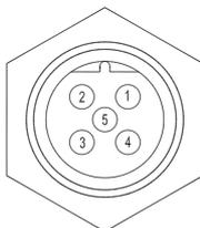
S3 connector (M12 5 pins B coded) line in view solder side MV
