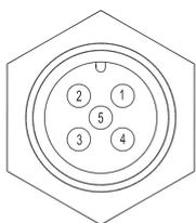
S3 connector (M12 5 pins B coded) line out view solder side FV
